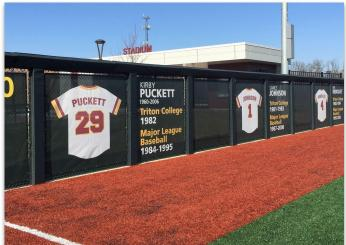
Custom padding panels are made of 3 inch thick polyurethane foam glued to a ¾ inch treated plywood backer and covered with an 18 oz. vinyl covering, a coated UV polyester fabric.
